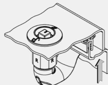
A further 90° rotation will pull the already latched cam 6.5mm [0.256] towards the frame: the seal is compressed, the door is latched and free of play.
