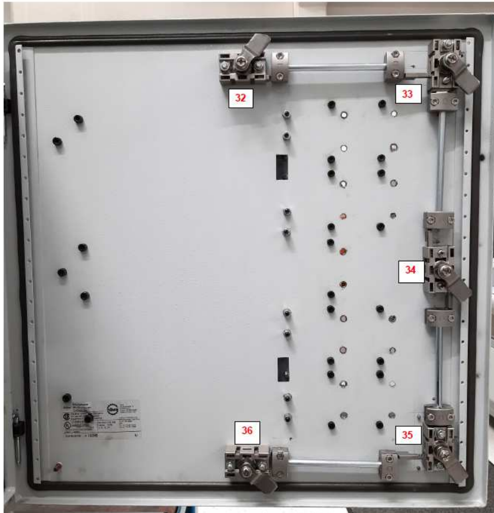
Abbildung 7: Arrangement of the test specimens
